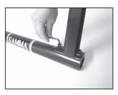
Align the holes in the leg flange with the matching holes in the lower column support post. Secure the leg with one FLAT HEAD cap screw through the upper hole, and one SOCKET HEAD cap screw through the bottom hole. Repeat this procedure for the three remaining legs.
