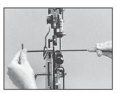
To tighten the braking mechanism, turn the set screw (A) counter clockwise by about 1/8 turn. Re-tighten the allen screw (B) on the back side of the tensioner frame and check for brake tightness. The tensioner should move freely along the track with the brake lever engaged and should hold tension with the brake lever released. If more adjustment is needed, repeat steps above until properly adjusted.
