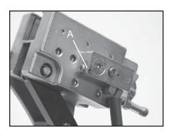
Loosen the 1.5 mm locking set screw (A) located on the side of the latching block as shown. The set screw is used to hold the adjustment screw in place.
