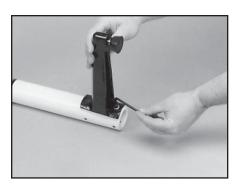
Secure the leg with one FLAT HEAD cap screw through the upper hole, and one SOCKET HEAD cap screw through the bottom hole. Repeat this procedure for the three remaining legs.
