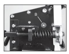
While holding the 5mm brake lever adjustment set screw (A), loosen the bolt (B) located on the back side of the tensioner frame with the 4 mm hex wrench.
