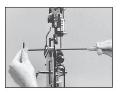
To tighten the braking mechanism, turn the set screw (A) counter clockwise by about 1/8 turn. Re-tighten the bolt (B) on the back side of the tensioner frame and check for brake tightness. The tensioner should move freely along the track with the brake lever engaged and should hold tension with the brake lever released. If more adjustment is needed, repeat steps above until properly adjusted.
