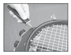
The machine includes the pathfinder stringing awl which creates a pathway between or around strings to make inserting a string through blocked grommets easier and quicker.
