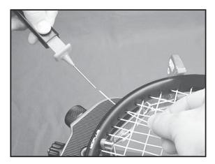
While holding the string, slowly pull the sheath out of the grommet hole to leave the free end of the string exposed.
