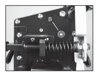
While holding the 6mm brake lever adjustment bolt (A), loosen the hex bolt (B) located on the back side of the tensioner frame with the 4 mm allen wrench.
