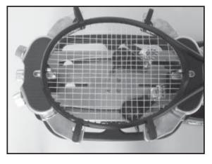
Once the final cross string is tensioned and clamped, tie off at the appropriate hole specified by the racquet manufacturer.
