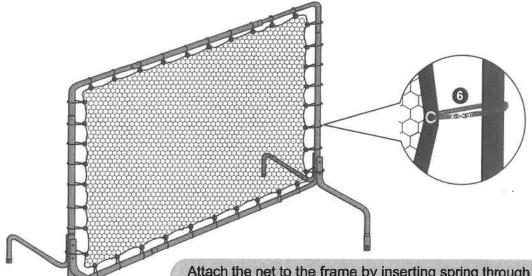
Attach the net to the frame by inserting spring through the eyelets in the net binding and around the frame tubing, using "S" hook to connect ends of spring. Begin by connecting a spring in the middle eyelet in each side and top of the net, then attach both sides and the bottom with a spring in each eyelet. Tilt the frame over to attach the top of the net.
