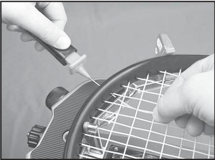
Once the awl is inserted, pull the handle of the awl outward while holding the tip section in place. This leaves the outer sheath in the grommet hole. Insert the end of the string into the outer sheath.
